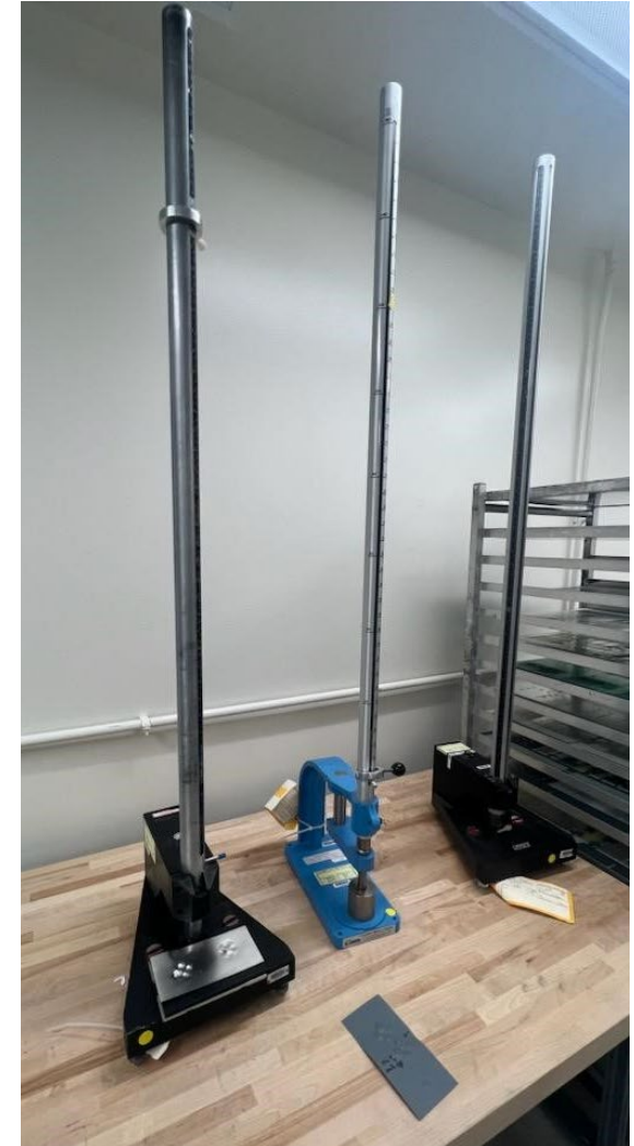
ASTM D2794 (GE Reverse Impact Test) Includes 0.5%, 1%, 2%, 5%, 10%, 20% 40% and 60% elongation
