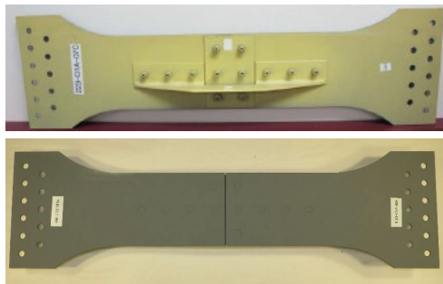
Structural Component Corrosion Simulation (SCCS) specimen
